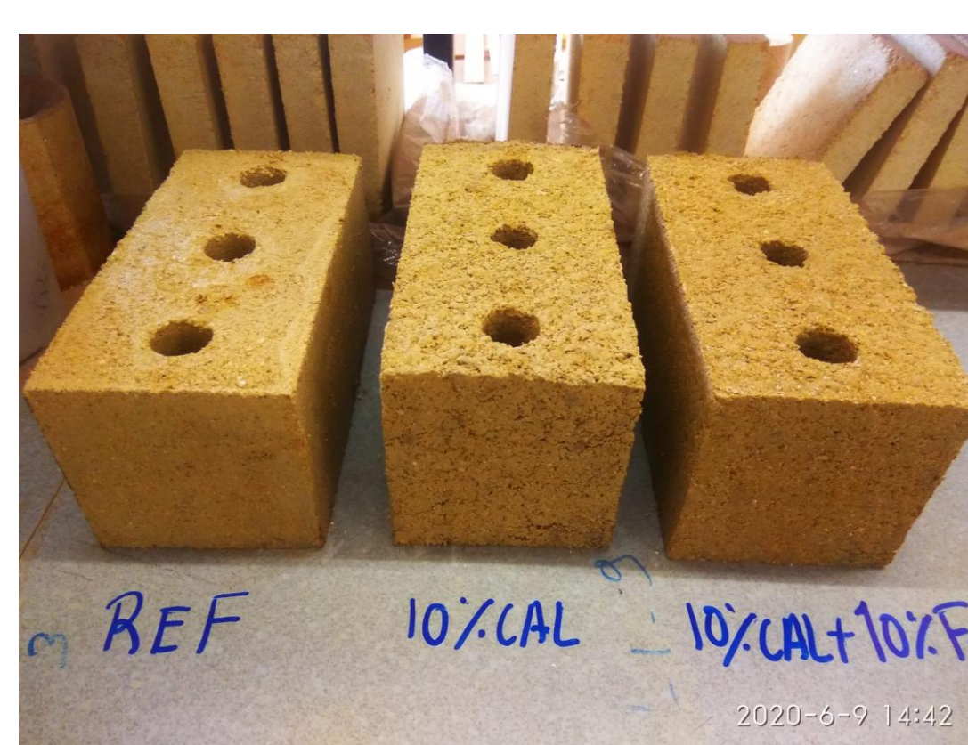
Fig. 11- Final blocks: block with soil, block with soil and 10% lime and block with soil, 10% lime and cigarette butts fibers
