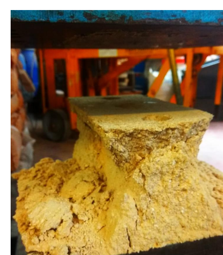
Fig. 12- Compression tests of the final blocks
