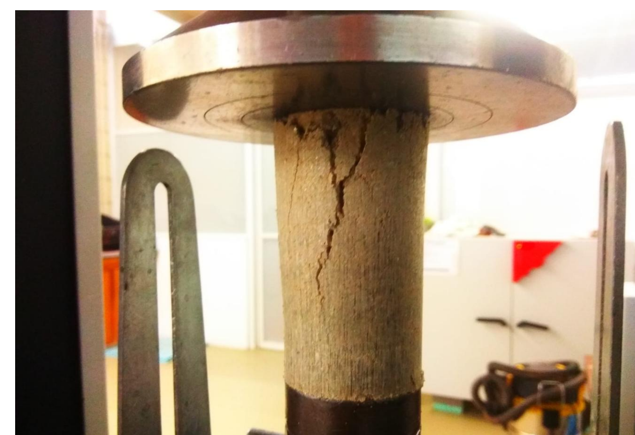
Fig. 7- Test pieces in the compression test
