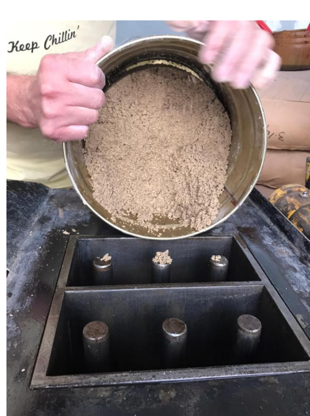
Fig. 9- Putting the mixture for the construction of the final test pieces in the mould
